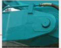
Integrated cast steel boom top
