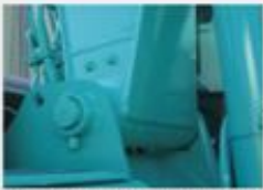
Cast steel boom foot boss
